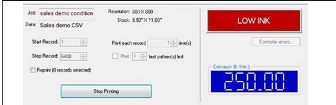
Image 8.3c: Printing Display Shows the Ink is Low and the Print Speed is Good
