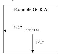
Although the camera system can learn many fonts for OCR, we recommend standardizing on OCR A or B.
