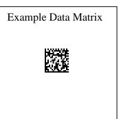
The Data Matrix code can be printed anywhere that the camera can see it of the inserter. The data in the data matrix code should only be the sequence number. Leading zeros are required to give the barcode a uniformed size though out the job.
